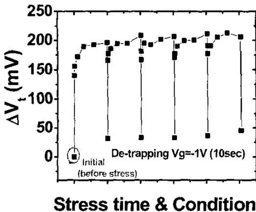
Fig. 4 Threshold voltage shift during five cycles of HC stress ( $V_g, V_d=2V/ 1000sec$ ) followed by the de-trapping step.
