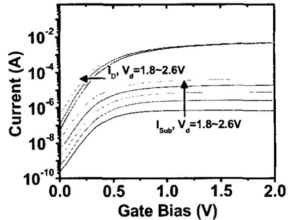
Fig.1 Dependence of  $I_d-V_g$  and  $I_{sub}-V_g$  curves on drain bias  $V_d=1.8\sim 2.6V$  in HfSiO/poly gate stack devices.
