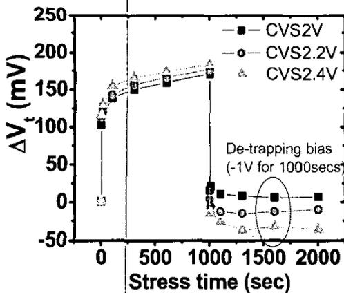
Fig. 8 Threshold voltage shift time dependence during CVS (1000secs) followed by the negative bias stress.
