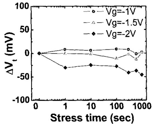
Fig. 5 Threshold voltage shift during the negative bias stress.
