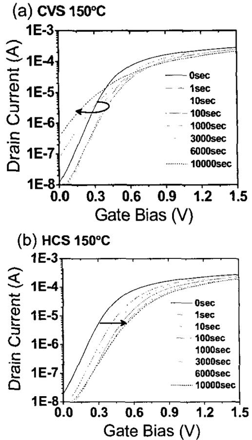
Fig. 9 Changes of the Id-Vg curve with stress time in HCS ( $V_g=V_d=2.4V$ ) and CVS ( $V_g=2.4V$ ) at 150°C
