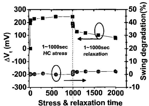
Fig. 2 Threshold voltage shift and subthreshold swing degradation (%) during HC stress ( $V_g=V_d= 2.2V$ ) and relaxation ( $V_g=V_d=0$ ) in HfSiO/poly-Si devices.
