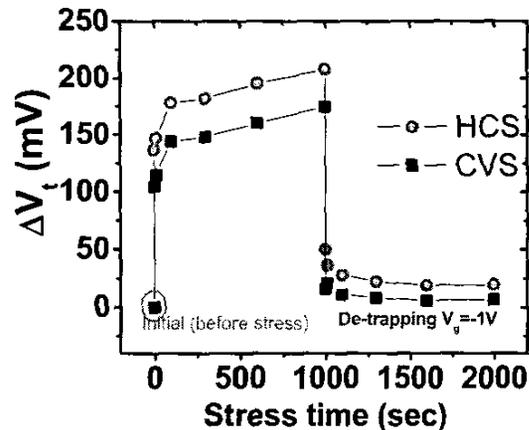
Fig. 6 Threshold voltage change during HC stress ( $V_g=V_d=2V$ ) and CVS ( $V_g=2V, V_d=0$ ) followed by the de-trapping step ( $V_g=-1V$ ).
