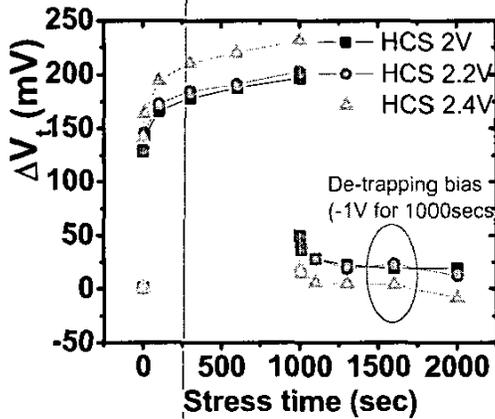
Fig. 7 Threshold voltage shift time dependence during HCS (1000secs) followed by the negative bias stress.
