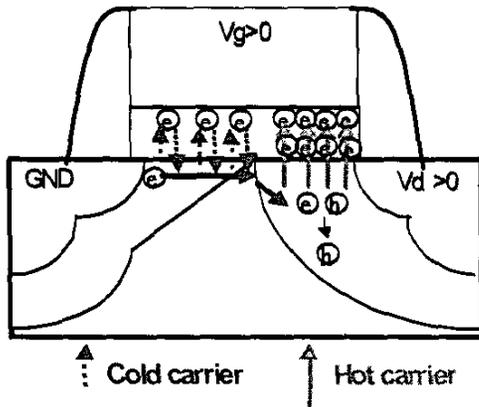
Fig.3 Schematic of the cold and hot carriers injection processes during the HC stress.
