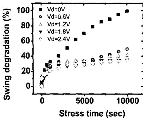
Fig. 10 Time dependence of the threshold voltage swing degradation at different drain voltages during HCS at 150°C ( $V_g=2.4V$ )
