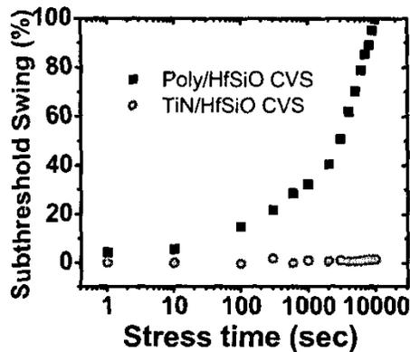
Fig. 11 Swing degradation during the constant voltage stress at 150°C in Poly vs TiN gate electrode transistors
