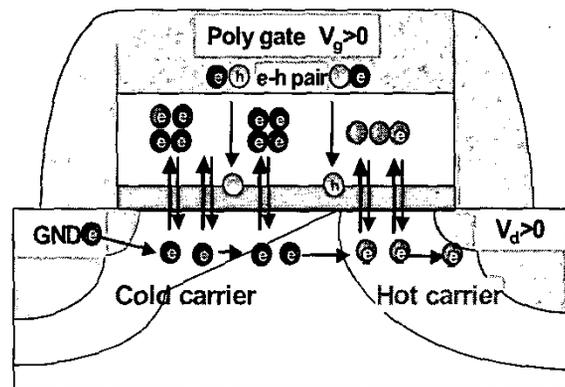
Fig. 13 Non-uniform hot carrier stress induced charge movements in high-k device with poly gate electrode.
